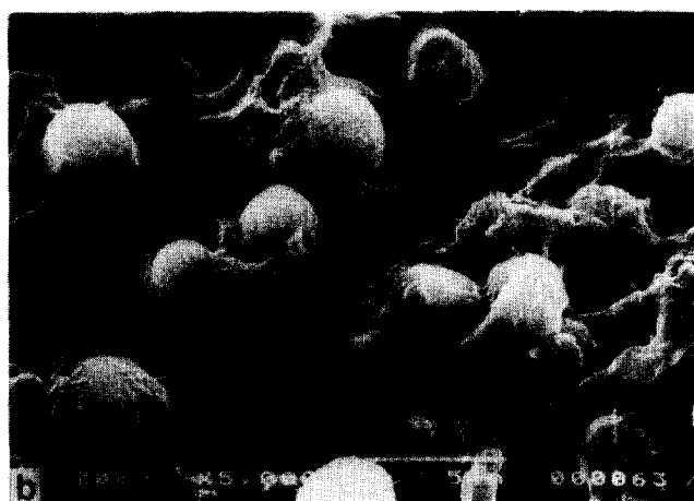
Figure 8 Scanning electron micrographs of blends microtomed and selectively etched at room temperature: (a) 25/75; (b) 50/50
