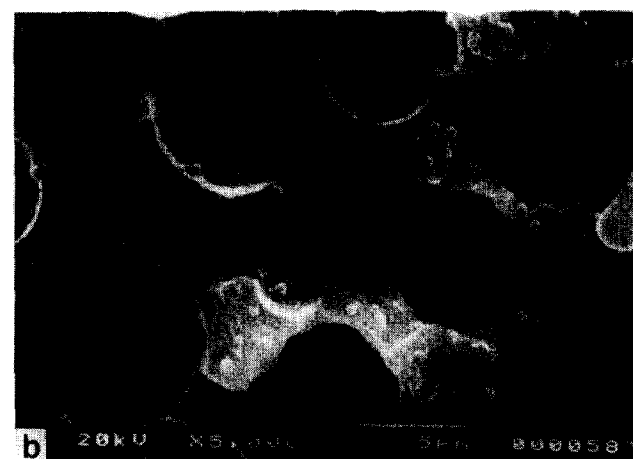
Figure 9 Scanning electron micrographs of blends microtomed at room temperature and selectively etched with boiling toluene: (a) 15/85; (b) 25/75
